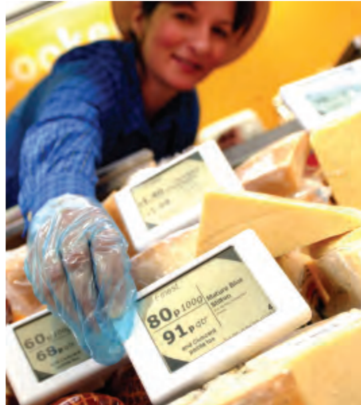
In partnership with ZBD Displays Ltd, our scientists have worked to develop the next generation of liquid crystal cell devices. These electronic displays allow retailers to make global changes to product information at the touch of a button.
