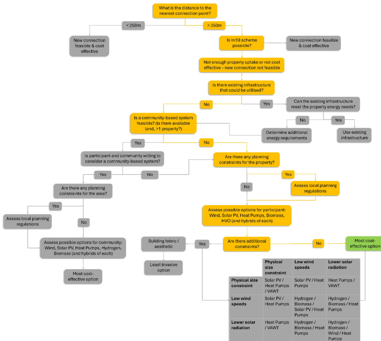
Figure 7: The decarbonisation assessment framework as applied to Story 2. Decisions made for Story 2 are highlighted in orange, the suggested decarbonisation option is highlighted in green.
