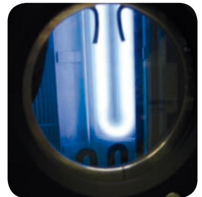
View through a viewport on the plasma of an active HIPIMS cathode (HAUZER).
