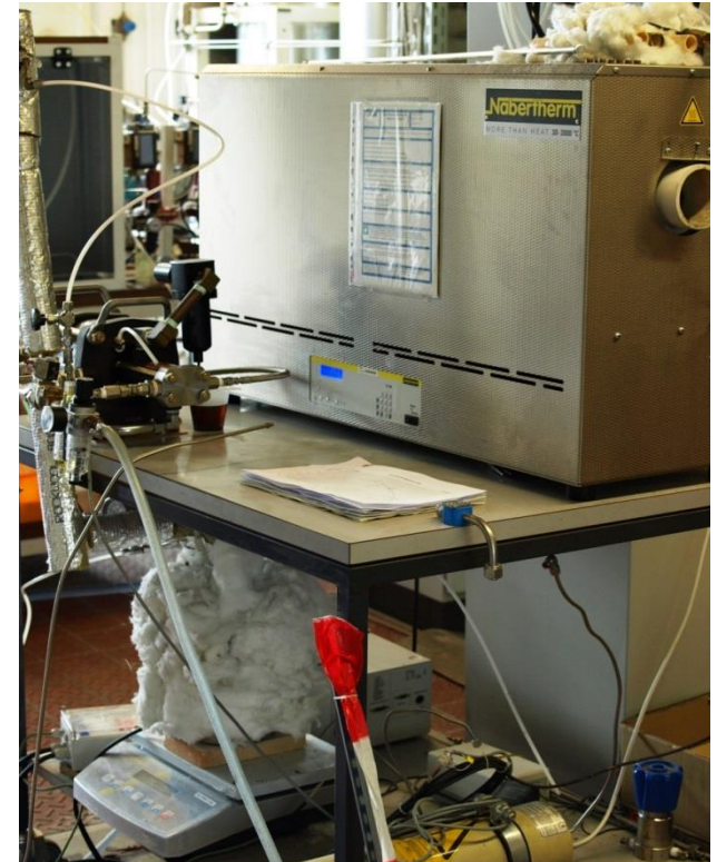
NABERTHERM R 100/750/12 furnace with a ceramic tube reactor
