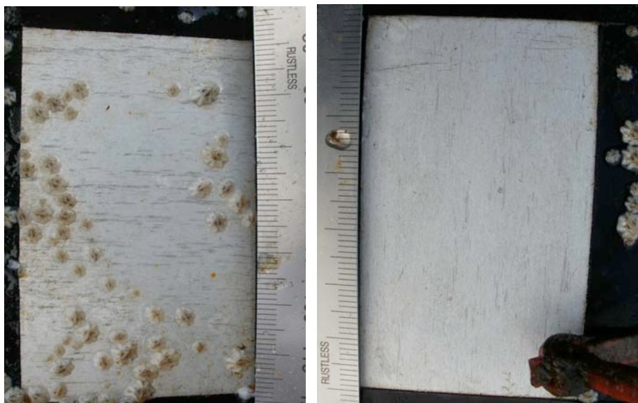
Figure 9. Comparison of barnacle settlement on sol-gel surfaces, abiotic (left) and biotic (right).
